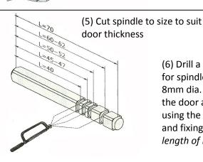
(6) Drill a 15mm dia. Hole for spindle and 3 no. 8mm dia. Holes through the door and fix OAD using the two cup washers and fixing bolts. (Reduce length of bolts if necessary)
