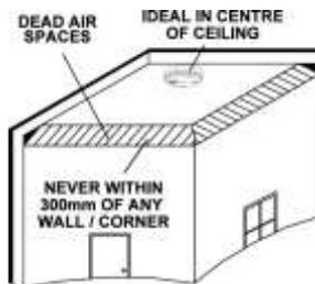
Place the alarm on the ceiling/wall and mark the screw holes. Drill with a suitable drill bit, insert the screw plugs and screw the alarm into position. Simply connect the battery on the alarm and slide into position on the mounting plate.
