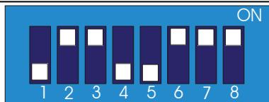
The address setting is binary, with the **ON** position being binary **0**, and the **OFF** position being binary **1**. Switch 8 is not used for setting the address, but sometimes has a device specific function. (check instructions that come with the device). **EG on sounder bases, switch 8 MUST BE ON.**
