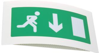
Comprising a white, stove-enamelled, zintec-coated sheet steel base, and fitted with a self-extinguishing legend panel, the ESS Light is designed for use on escape routes and final exits. It conforms with the 850°C hotwire test, as defined by ICEL.
