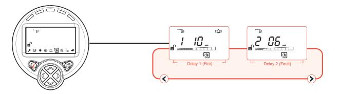
On entering this option Delay 1 (Fire) is displayed; Delay 2 (Fault) is accessed by using the Left & & Right arrow keys, which toggle between the two delays. It is not possible to set the Delay to Fire to less than the Delay to Fault.
