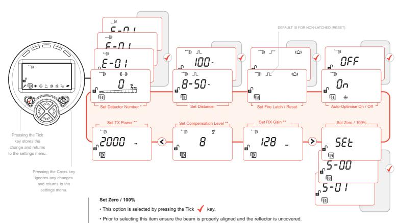
• S-00 (Step 0) is displayed, the installer MUST cover the reflector and then press the Tick 🗸 key whilst it is still covered.
