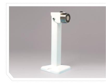
This rugged, versatile design of door magnet can be used for many different door holding applications. With the magnet set as shown in the photograph, the door holder can be floor mounted or ceiling mounted. Turn the magnet through 90° and the door holder is in wall mounting configuration.
