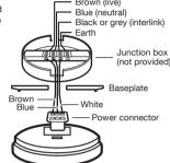
If desired, the alarm can be interconnected with up to 11 other smoke (SW1), heat (HW1) or carbon monoxide (CW1) alarms from
