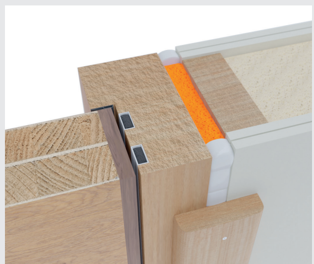
Image B – FD90 & FD120 foam with intumescent acrylic sealant cap of 10mm minimum.
