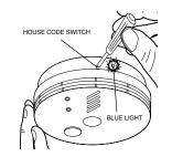
Check the communication by pressing the test/hush button for up to 20 seconds on each unit in turn. The red light will flash, the Alarm will sound and blue light on the RadioLINK Base sidewall will illuminate continuously for around 3.5 seconds. All other Alarms should sound (this may take up to 20 seconds).
