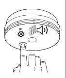
To test an individual Alarm press and hold the test button until he horn sounds and the red light flashes. This will ensure that the sensor, electronics and sounder are working.
