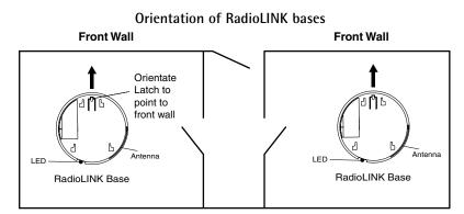
Orientate all RadioLINK bases in the same direction
