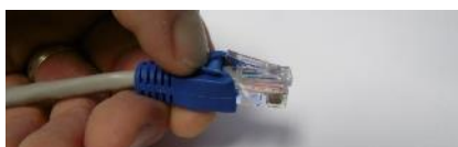
Pull boot back to access lock clip
