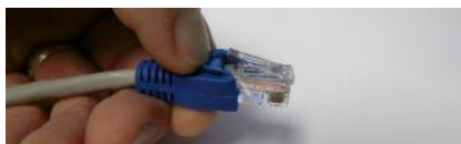
Pull boot back to access lock clip
