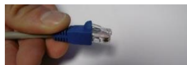
Slide boot back over lock clip
