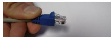
Slide boot back over lock clip
