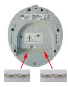
To ensure proper operation, using your finger press lightly on each of the four pins in turn. Each pin will push back into the SAM 500P. Check that each pin springs back after it has been released.
