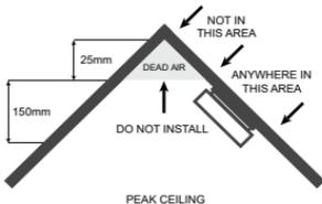
These alarms should be installed no more than 150mm vertically below the apex of a pitched ceiling. Where the depth from apex to eaves is 600mm or less the ceiling should be treated as flat.
