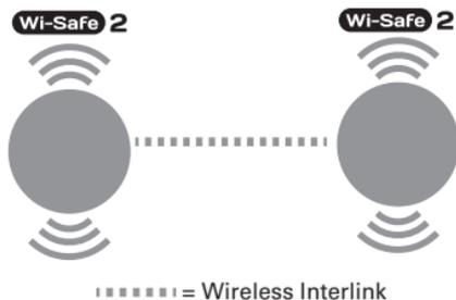
Wi-Safe 2 enables wireless communication with any other product with Wi-Safe 2 technology inside. A wireless transceiver inside every alarm communicates with others by continuously sending and receiving wireless signals otherwise known as a 'meshed network'. When one alarm detects CO the wireless module inside sends a radio frequency signal to all the connected alarms, ensuring almost
