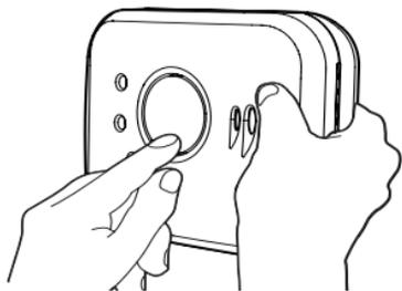
The red LED on Alarm 2 will flash to indicate that it has been 'learned-in' successfully. If the test button is not pressed quickly enough, the 'learn-in' process will fail. If this happens, repeat the process. To complete the installation fit Alarm 2 into position.
