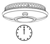
**3.** During the reduced sensitivity reset cycle, the red LED on your alarm will continue to flash more rapidly than normal, approximately once every 10 seconds.
