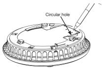
The red LED next to the learn button will flash briefly then light up for approximately five seconds to show that it is ready to receive the "learn in" signal. During these five seconds you will need to briefly press the test button on Alarm 1 to wirelessly interlink the two alarms.
