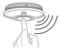
**2.** Your alarm will silence and enter into a reduced sensitivity reset cycle for approximately 10 minutes.
