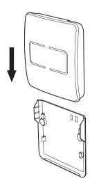
To complete the installation simply slide the control unit onto the bracket. The control unit is now part of the whole network.
