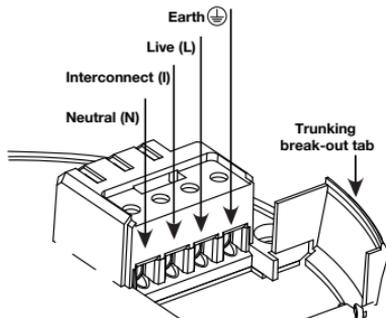
**WARNING:** Mixing the Live and Neutral connections when interconnecting alarms will damage all the alarms. DO NOT use the Earth wire for the interconnect connection.
