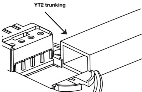
Either feed the wire through the hole in the base plate or through the YT2 trunking.
