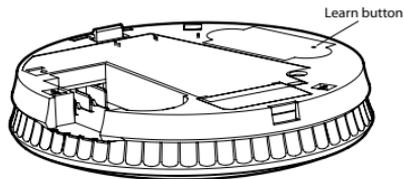
Using a ballpoint pen briefly push and release the 'learn button' on the back of Alarm 2. The red LED next to the learn button will flash briefly then light up for approximately five seconds.
