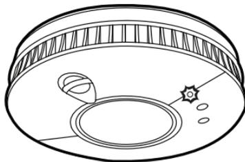
Check that the green LED is on and that the red LED is flashing once approximately every 45 seconds. The LEDs are located on the front of the alarm.
