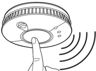
During the reduced sensitivity mode the red LED on your alarm will continue to flash more rapidly than normal, approximately once every 10 seconds. Only use the alarm silence function after making sure that there is no fire emergency situation. Do not block the vents on the alarm or disable the alarm in any way, as this will remove your protection.
