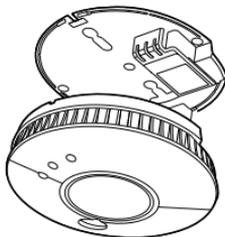
Line up the alarm with the base plate and gently apply pressure until the alarm clicks into place. Switch on the mains electricity supply.
