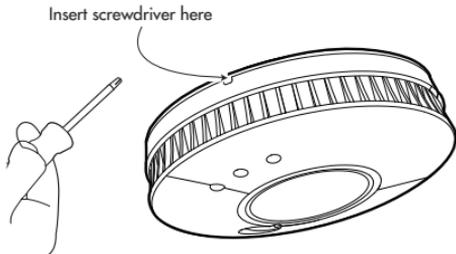
Push the screwdriver in and the alarm should fall free from the base plate. Please be aware that the alarm will fall as soon as pressure is applied to the screwdriver, be prepared to catch it.
