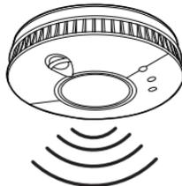
An audible alarm consisting of two cycles of three loud beeps should occur and then stop automatically. The red LED on the alarm will flash rapidly during the audible signal.
