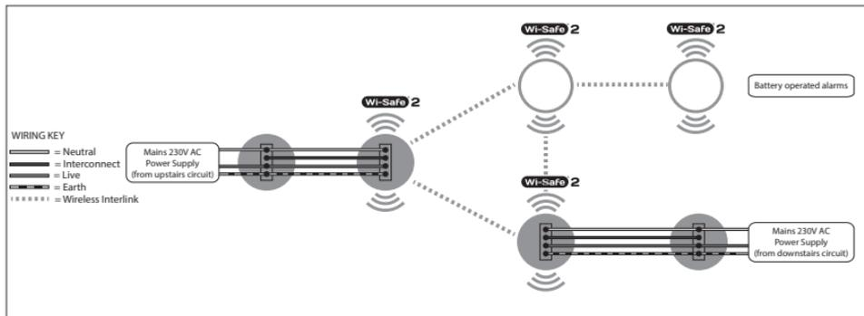
**Make sure there is only one wireless connection into each wired network.** For example if you have a hardwired network upstairs and a wireless network downstairs only one of the hardwired products should be linked into the wireless network, connecting both systems.
