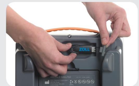
Plug a memory stick into the USB port to download rescue event data, upload a new configuration, or upgrade software.
