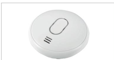
**Why optical?** Replacing the older ionisation technology, optical smoke sensors are less susceptible to false alarms caused by normal household fumes like bathroom steam, dust, or normal cooking vapours – even the toaster. Optical sensors are also quicker to react to slow, smouldering fires often associated with electrical equipment and furniture.
