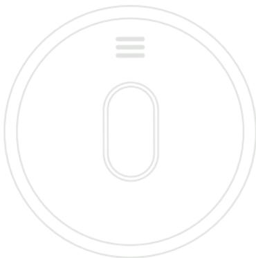
During standby, the LED will flash every 50 seconds to indicate normal operation. When in alarm mode the LED flashes approximately once per second and the alarm enters into one of the alarm patterns described in the Alarm Signals section.
