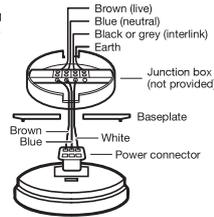
**2c** Push and twist the alarm clockwise onto the base plate. Turn the electricity supply back on and check that the green LED is on.
