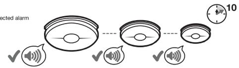
On an interconnected network, only the alarm that senses the fire will sound and flash its LED. Other connected alarms will sound a warning but will not flash their LED. Do not connect more than 11 other devices.
