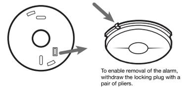
To enable removal of the alarm, withdraw the locking plug with a pair of pliers.
