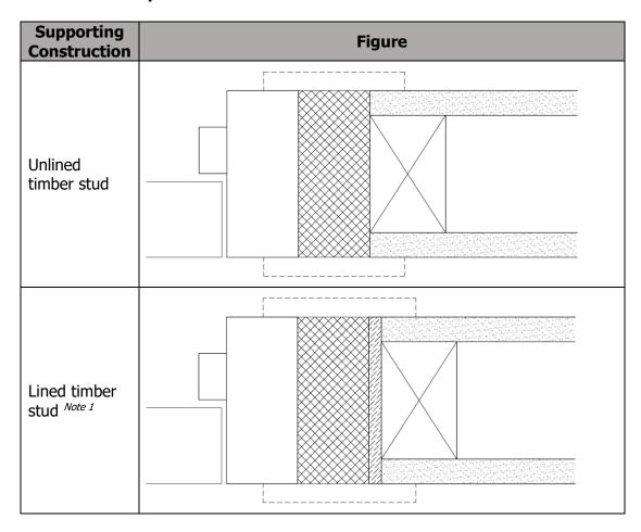
Note 1 The lining of the timber stud must use the same board, of the same thickness, as used in the construction of the wall.
