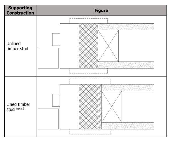
Note 2 The lining of the timber stud must use the same board, of the same thickness, as used in the construction of the wall.
