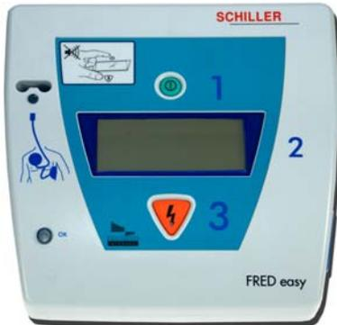
The FRED easy with silent mode option is intended for locations where a quick transferral to a hospital cannot be guaranteed. If in Silent mode a change in the cardiac rhythm is detected the device reactivates the AED mode and the user will be prompt to check the patient.
