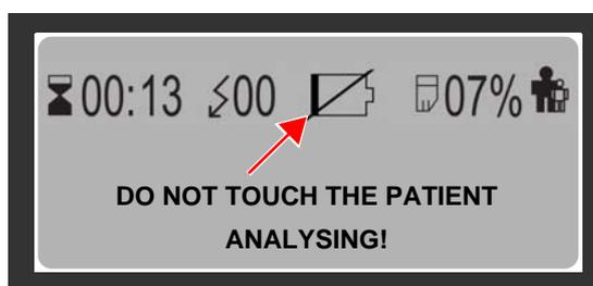
**Fig. 3.4** Low battery capacity
