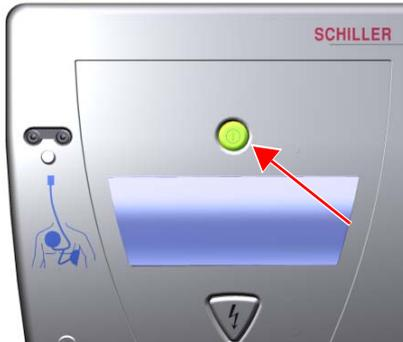
**Fig. 2.1** Button to switch the device on and off, and to start the analysis (only in semi-automatic operation)
