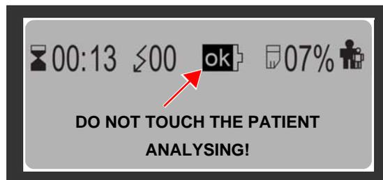
Fig. 3.2 Sufficient battery capacity
