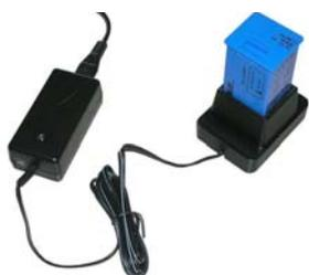
Fig. 6.2 NiCd battery charging unit
