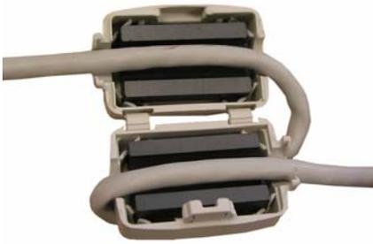
**Fig. 5.6** Installing the cable within the ferrite core
