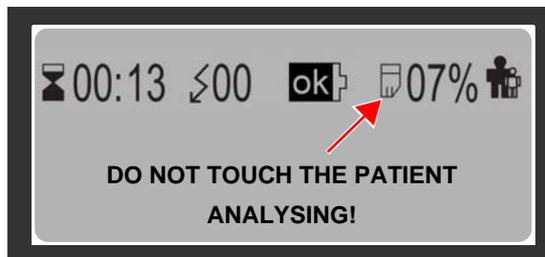
**Fig. 5.2** SD card inserted
