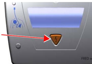
Fig. 4.8 Button to deliver the shock
