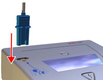
Fig. 4.3 Inserting the connector into the port
