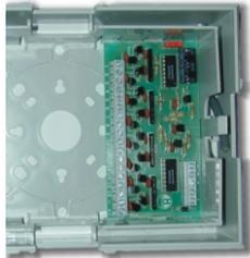
The MG020000 uses serial data from a master unit to provide up to 16 outputs capable of switching up to 500ma per zone (subject to psu limit). Six outputs follow the annunciator LEDs. Six further outputs switch on alarm condition and restore on reset. Two outputs follow the integral sounder and global relay. Two outputs are not nominated. These cards will fit into the Multiguard back box as shown. Dimensions 135 x 67 x 15 (mm)
