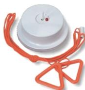
The S1631 pillow push is supplied with 2m of cable. It is a non latching device with a normally open contact that closes when pressed. It can only be used with an S1663P electronic call point as part of a Multiguard nurse call system.
