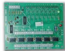
The MG030000 takes the serial data from a master unit to provide six relay outputs with voltage free DPCO contacts (1A/30vdc resistive). The activation of these relay outputs is dependant upon the software configuration of the master unit.
