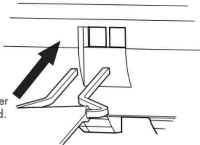
**i NOTE:** If the disabling tab is no longer available then the clip can be replicated by opening out a thin metal paper clip into a U-shape.
