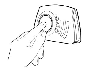
Test the sounder, power pack and circuitry by pressing and releasing the Test/Silence button to confirm that the detector is operating properly.
