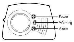
Your cold alarm is designed to give a series of visual and audible warnings when the temperature falls. If only the Power LED is flashing once per minute then the temperature in the room is 18°C or above. Other temperatures below this will result in one of the following indications:
