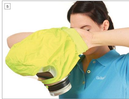
5 Widen the neck seal and pull the hood over your head. The inner head harness automatically adjusts to your head. Ensure that nose and chin sit comfortably in the half mask and that all hair is tucked into the hood.
