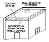
Place the alarm on the ceiling/wall and mark the screw holes. Drill with a suitable drill bit, insert the screw plugs and screw the alarm into position. Simply connect the battery on the alarm and slide into position on the mounting plate.
