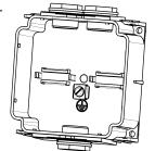
vertical plane. The back box can be mounted with either the single or the double entry holes at the top.
