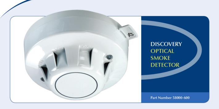
The Discovery Optical Detector has a white moulded polycarbonate case with wind-resistant smoke inlets. The indicator LEDs are colourless when the detector is in quiescent state and red in alarm. Within the case is a printed circuit board which, on one side, has the light-proof chamber with integral gauze surrounding the optical measuring system and, on the other, the signal processing and communications electronics.
