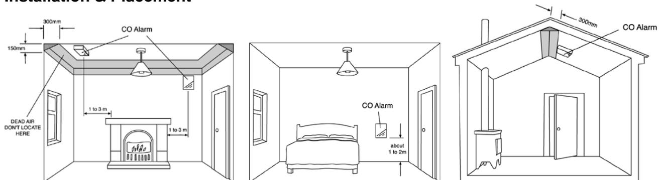
To mount onto a wall or ceiling, simply remove the battery compartment and mark the position of the two mounting holes. Drill two holes using a 6mm drill for the plastic plugs (supplied) and screw the unit home with the screws supplied
