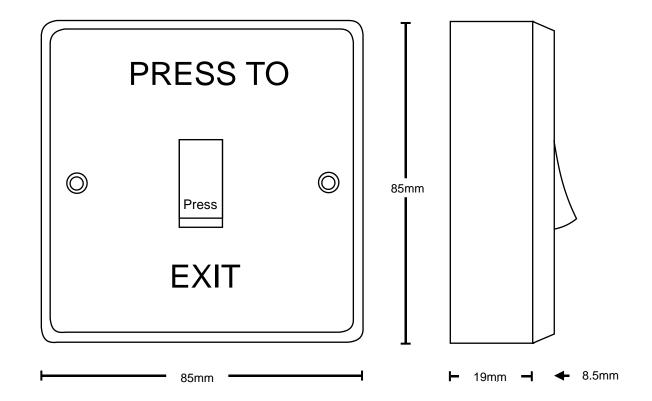
Surface box seperate to allow surface or semi flush mounting. NO, C and NC Contacts
