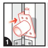
Offer up the fitting jig to the door leaf with the lip on the knuckle side of the door just below or above the middle hinge. The centre line should always be 22mm from the knuckle side of the door.
