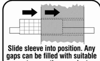
mortar, mastic or sealant
