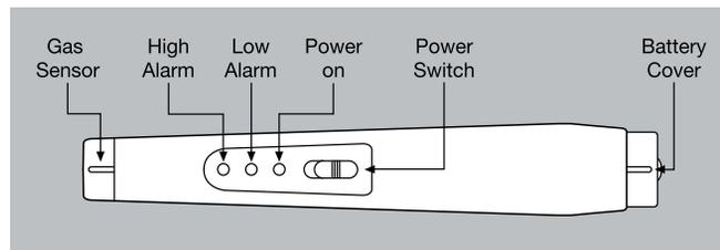
Simply check the suspected area by pointing e<sup>2</sup>sense close to the source. If gas is present the alarm will sound and the yellow LED or the red LED will light up according to the concentration of gas. It couldn't be simpler.
