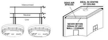
Be very careful about correctly wiring the alarms as mixing Live and Neutral will blow/damage interconnected alarms.
