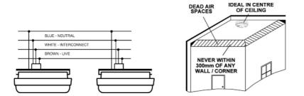
Be very careful about correctly wiring the alarms as mixing Live and Neutral will blow/damage interconnected alarms.
