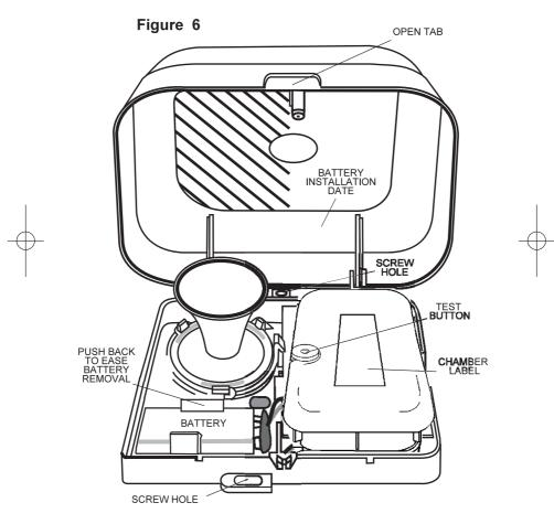
The Smoke Alarm is battery operated and needs only wiring, if the Inter-Link facility is being used.
