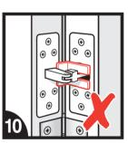
Installing the closer the wrong way will result in failure and is not covered by any warranty or guarantee. Note: The 'Astra England' stamp may be upside down, depending on the handing of the door.
