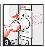
Drill the hole for the closer body using the auger bit. Do not drill to excess, the door control should be a snug fit.
