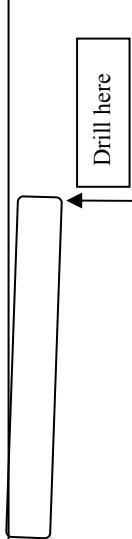
Similarly, if mounting on a wall allow a 1 - 2 degree slope in the horizontal plane and drill a 1mm hole in the lower edge of the diffuser to allow any condensation to escape.
