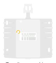
Turn the screwdriver anti-clockwise 5 degrees (A small adjustment is equivalent to a large alteration in sensitivity).
