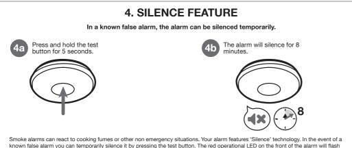
known false alarms van teacher of cooking turnes of other interpretering situations. The red operational LED on the front of the alarm will falsh behind the plastic surface once every 8 seconds to show that it is in Silence mode. Your alarm will automatically return to full sensitivity after 8 minutes. The alarm will sound continuously and the Red operational LED flashes behind the plastic surface every second when the alarm senses smoke.
