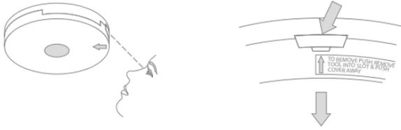
Locate the directional arrow on the front face of the alarm, the removal slot is located directly above the arrow.
