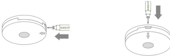
Insert the supplied removal tool approx. 1cm into the alarms removal slot and lever it down gently.
