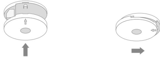
Place the alarm on the base, slightly offset from the centre and slide in the opposite direction to the arrow on the cover until it "clicks" into place.
