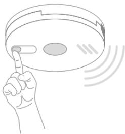
Press and hold the test button for 10 seconds, the alarm should sound loudly.
