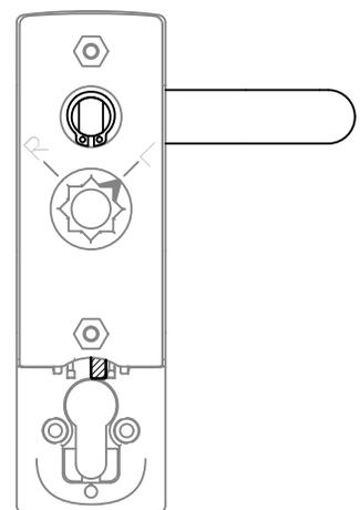
USING A 2.5MM ALLEN KEY LOOSEN THE GRUB SCREW AND REMOVE THE HANDLE, REPLACE AS SHOWN AND RETIGHTEN THE GRUB SCREW
