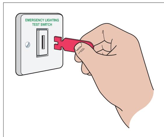
Test facilities often take the form of a 'fishtail' key (see Figure 64) inserted in a special switch either near the main fuse board or adjacent to relevant light switches.
