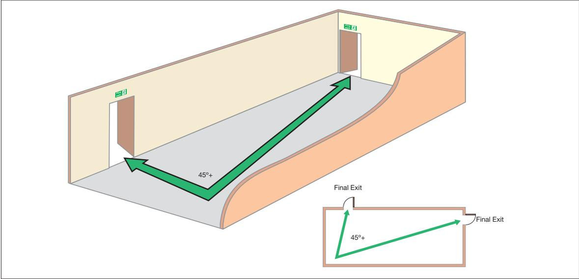
Figure 49: Ground floor premises with more than one exit
