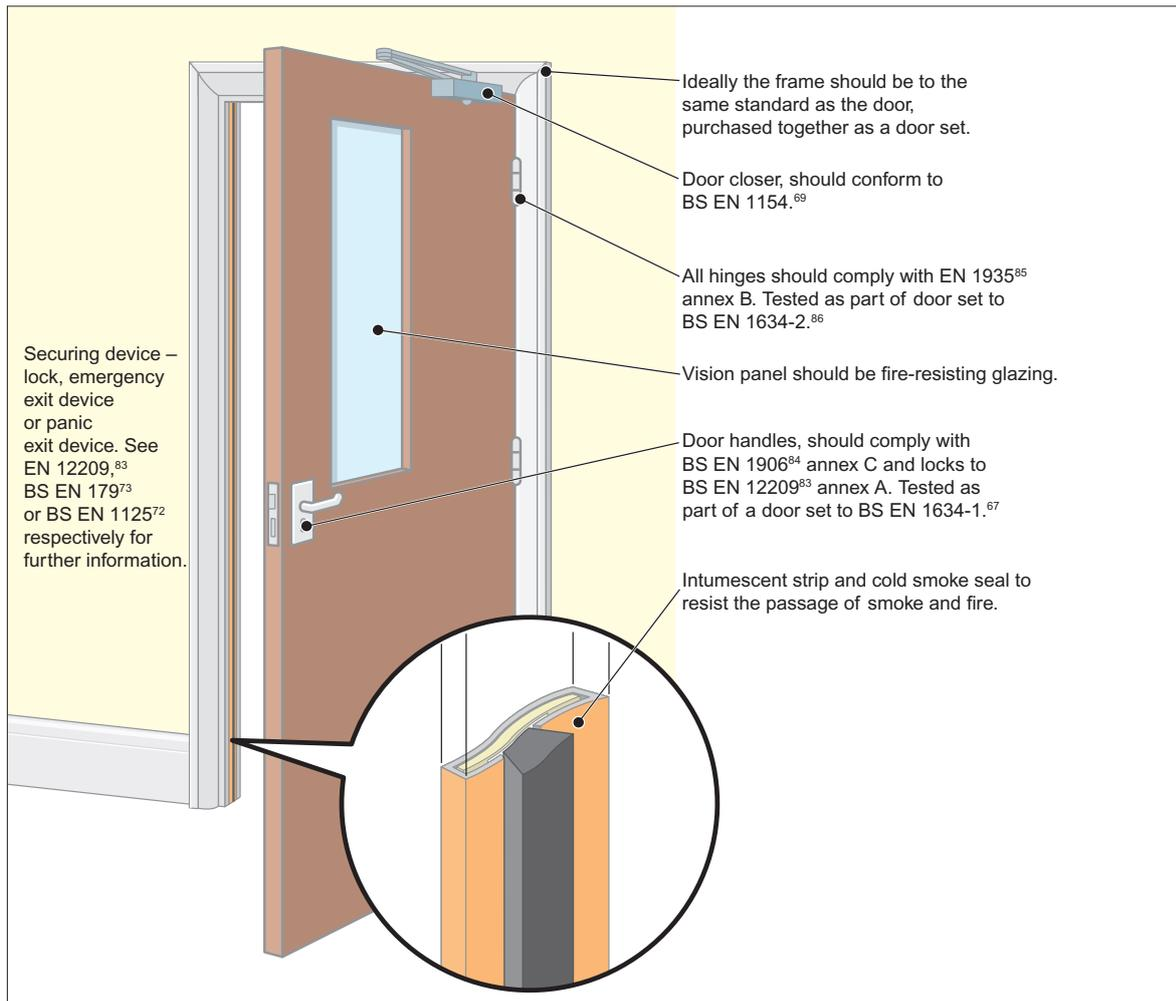
Fire-resisting doors are necessary in any doorway located in a fire-resisting structure. Most internal doors are constructed of timber. These will give some limited protection against fire spread, but only a purpose-built fire-resisting door that has been tested to an approved standard will provide the necessary protection. Metal fire-resisting doors are also available and specific guidance for these follows.
