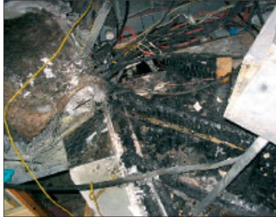
Figure 19: Fire in an air-handling unit (electrical) (courtesy of Network Rail)
