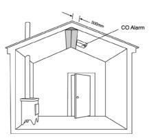
To mount onto a wall or ceiling, simple remove the battery compartment and mark the position of the two mounting holes. Drill two holes using a 6mm drill for the plastic plugs (supplied) and screw the unit home with the screws supplied
