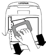
Hold down the left side of the electrode packet with one hand and pull the red packet handle down with the other. The electrode packet tears open.
