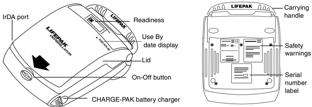
**Figure 2-1** Outside Controls, Indicators, and Labels
