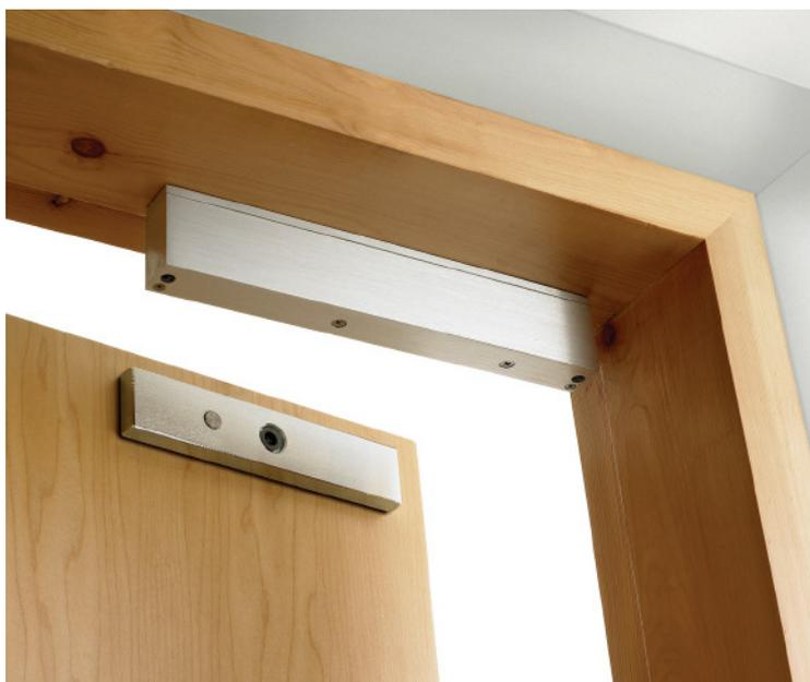
*For outward opening doors the magnet is mounted as shown on underside of the head frame with the armature plate to the closing door face.*
