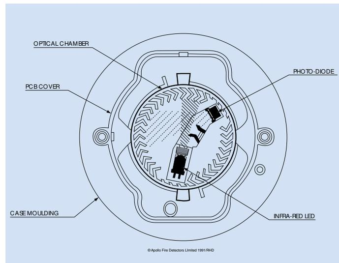
Fig.2 Top section, Series 65 Optical Smoke Detector
