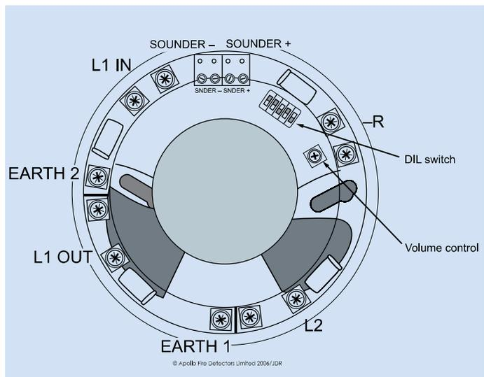
**Fig.8** Wiring diagram of Series 65 Sounder Base
