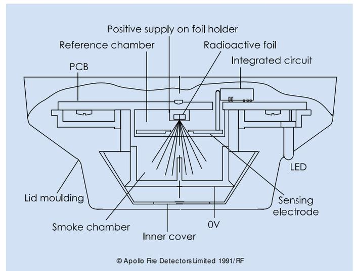
Fig.1 Side view, Series 65 Ionisation Smoke Detector
