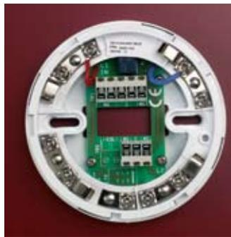
**Auxiliary Relay Base, 45681-246**, provides two sets of volt-free changeover contacts to facilitate the switching of a remote LED or other auxiliary device.
