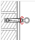
Tighten locking nut on eyebolt with a spanner. Do not over-tighten!
