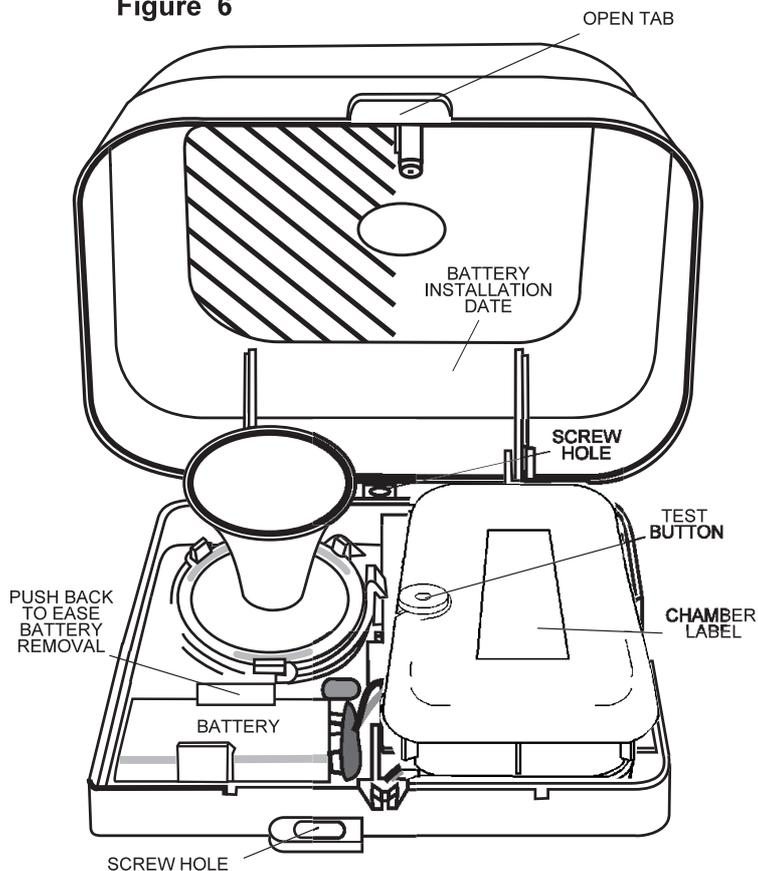
The Smoke Alarm is battery operated and needs only wiring, if the Inter-Link facility is being used.
